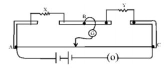
When a resistance of  $15\Omega$  is connected in series with 'Y', the null point is found to shift by 10cm towards the end A of the wire. Find the position of null point if a resistance of  $30\Omega$  were connected in parallel with 'Y'.
